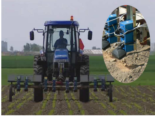
Figure 1: The camera unit consisted of camera combined with halogen lamp. During image acquisition were eight such units mounted in front of a tractor.
