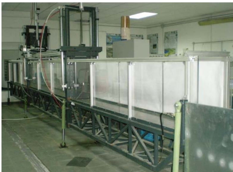
Figure 3. Flume used for experimental measurements.
