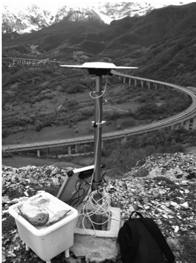
Fig. 3. Forced centering pillar used in the local GPS network survey (image by Livio Pinto)
