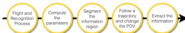
Figure 13. Methodology to build a 3D map of the material inside the trailer during a loading process using a forage harvester.
