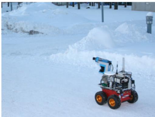
Figure 10. Tjorven, our mobile robot platform. In addition to the laser scanner used for 3D mapping, it is also equipped with a digital camera, an array of sonars, an omnidirectional camera (not shown here), and a differential GPS system.
