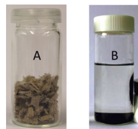
Figure 7. Holocellulosic fractions derived from two different Ni-catalysed up-stream processes: A) Raney-Ni catalysed removal of lignin from Poplar wood chips (pulp conducive to further downstream processing [198] ), and B) Ni/C catalysed removal of lignin from Birch wood saw dust (pulp not conducive to enzymatic hydrolysis [281] ). Image (A) reproduced with permission from Angew. Chem. Int. Ed. 2014 , 53 , 8634–8639; Angew. Chem. 2014 , 126 , 8778–8783. Copyright 2014 John Wiley and Sons. Image (B) reproduced with permission from Energy Environ. Sci. 2013 , 6 , 994–1007. Copyright 2013 Royal Society of Chemistry.
