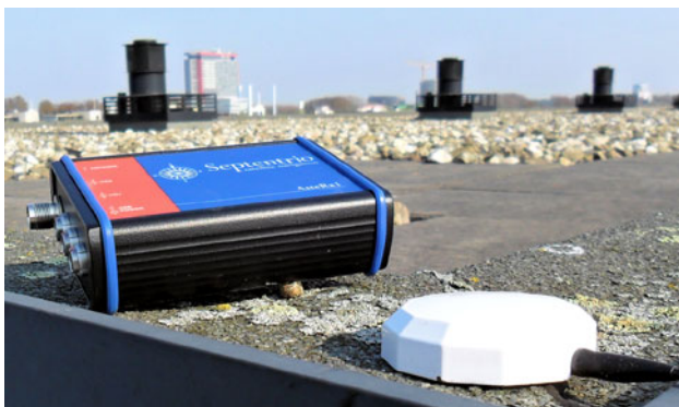
Fig. 3 The Septentrio AsteRx1 single-frequency receiver with the Aero 575-70 patch antenna
