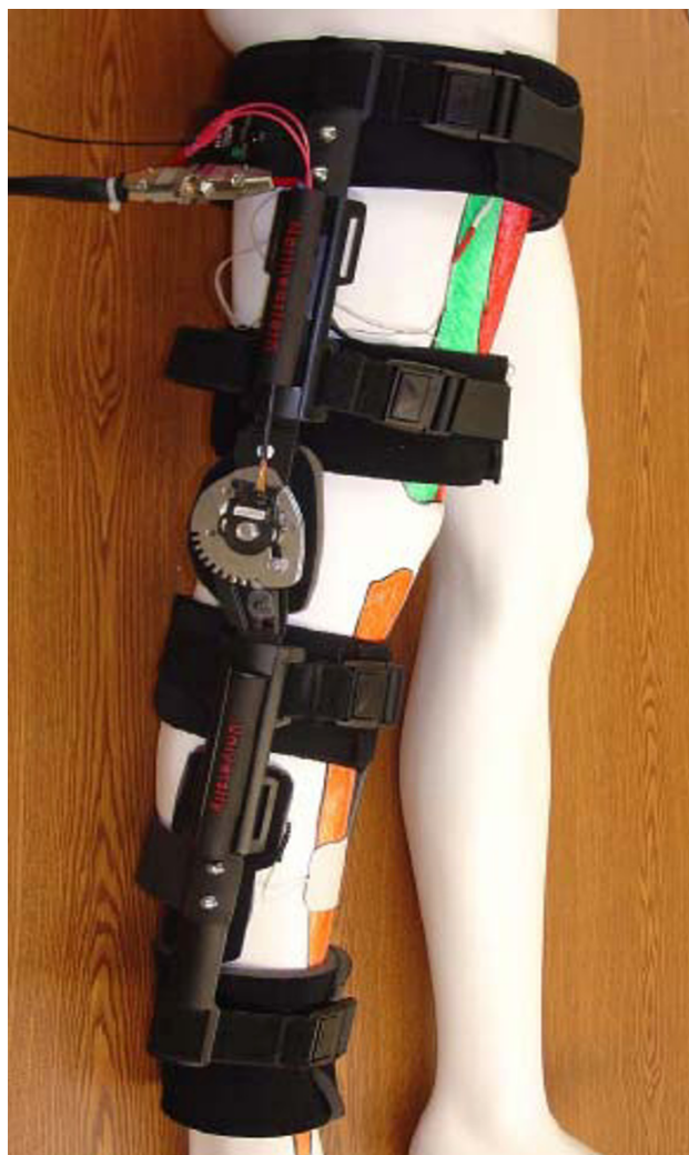
Figure 12 Electrical stimulation and biofeedback knee device.
