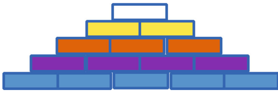
Fig. 7 A shift-invariant, scalable operator. Processing is from the bottom (input) to the top (output). Each layer consists of identical blocks, each block has two inputs and one output; each block is an operator H_2 : \mathbf{R}^2 \mapsto \mathbf{R} . The step of combining two inputs to a block into one output corresponds to coarse-graining of a Ising model.
