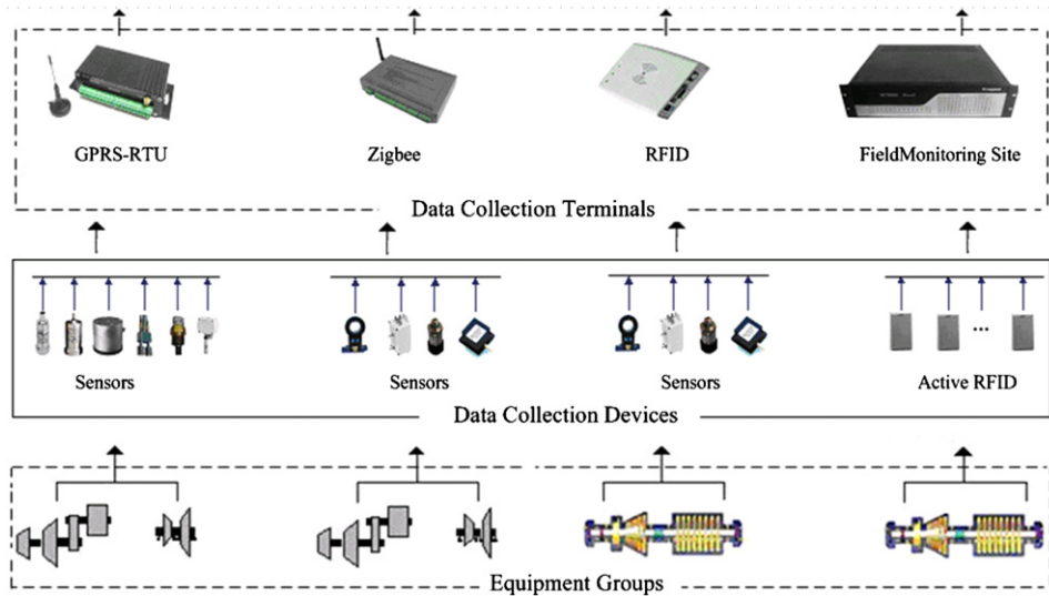
Fig. 3. Composition of sensor-monitoring layer.
