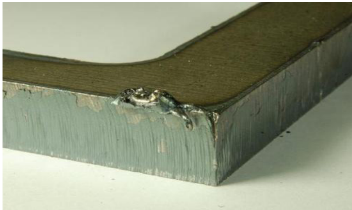
Fig. 2. Example of quality defects on a workpiece
