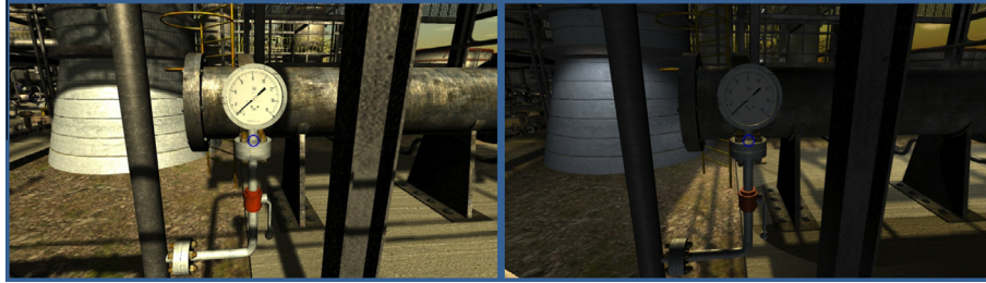
Fig. 4. Pressure gauge at neutral daylight conditions (no refraction, optimal readability – left) and at the sunset (diminished reading capability – right).
