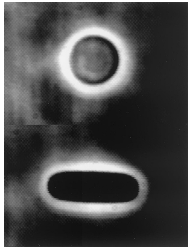
FIGURE 12 An example of an RBC stretched beyond the linear regime. The top part shows the undeformed cell trapped at 5 mW with a radius \rho = 3.36 \pm 0.05 \mu\text{m} . In the lower part, the cell is stretched with a peak stress \sigma_0 \approx 2.55 \pm 0.10 \text{ Nm}^{-2} to \rho = 6.13 \pm 0.05 \mu\text{m} along the beam axis, an increase of 82 \pm 3\% . After reducing the power, the cell returned to its original shape.
