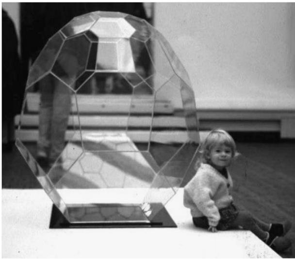
Figure 12 Facetted shell structures with three-way vertices: in these structures, loads are carried via the membrane stresses in the facets and the distributed shear along the edges (Bagger et al., 2007a).
