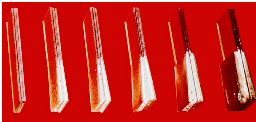
Figure 4 Clear intumescent interlayer: when exposed to fire, it turns into an opaque fire shield (AGC, 2008).
