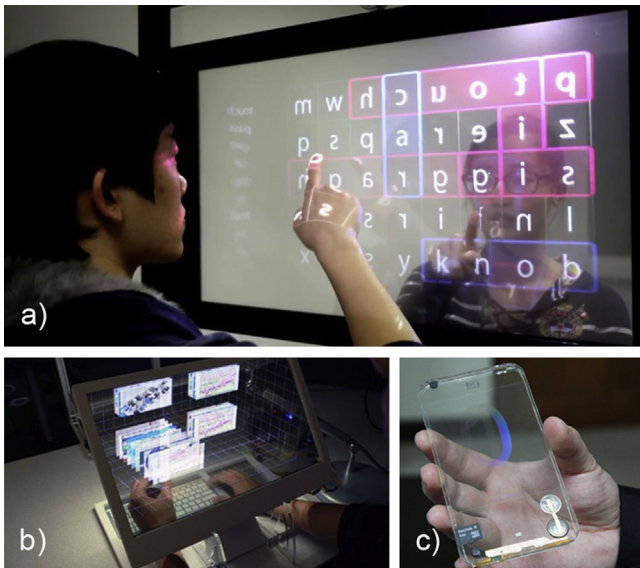
Figure 26 Transparent double-sided screens: the transparent types of electronic components make it possible to produce transparent double-sided screens (Vyas, 2014) (a), (Futuristicnews) (b), and (Scott, 2013) (c).
