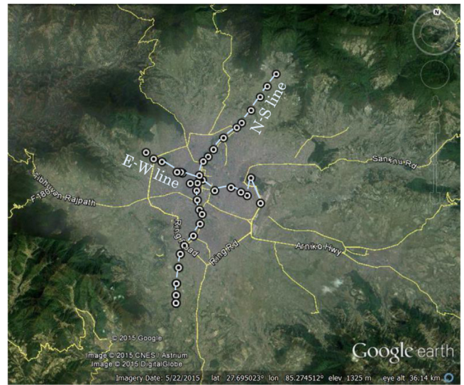
Fig. 9. Microtremor measurement arrangement along two lines across Kathmandu Valley, NS Line and EW Line (after Kukidome et al., 2009).
