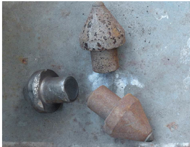
Fig. 8. Image of the actual damaged bowl-mill rolls after failure.
