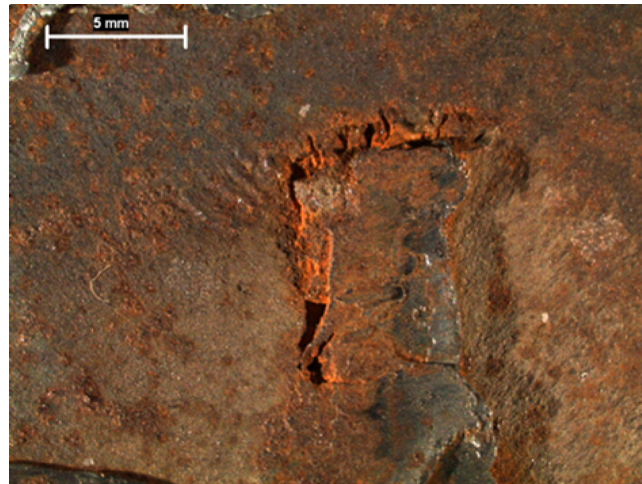
Fig. 4. Possible final fracture region on gear box side fractured surface.
