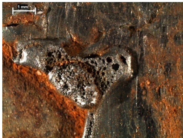
Fig. 3. Molten and re-solidified regions on the gear box side fractured surface.
