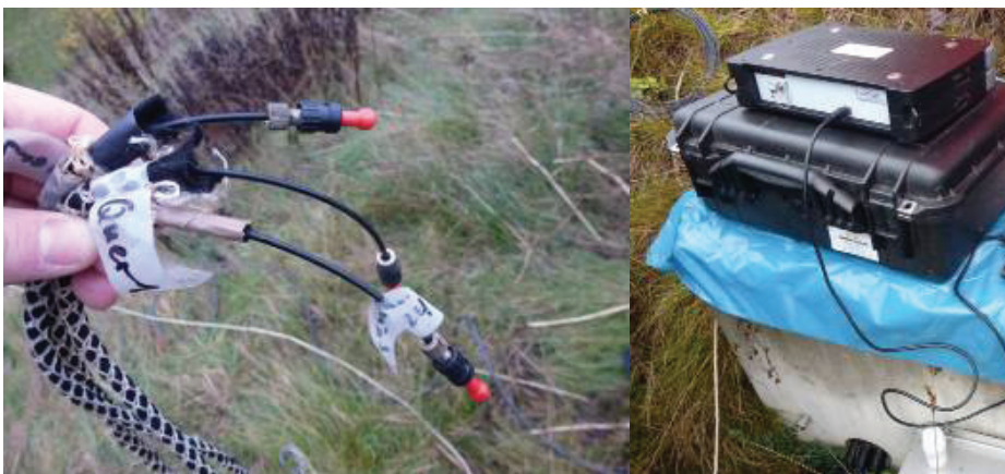
Fig. 11. View of the sensors and acquisition unit at the test side.
