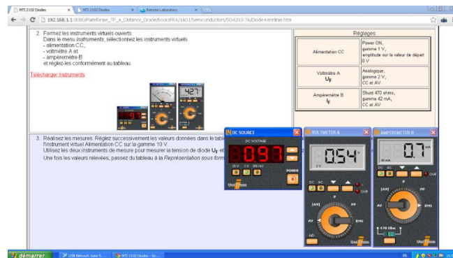
Fig. 2. Interface of the measurement of the diode voltage U_F and the diode current I_F by switching the virtual instrument on the DC power on the 10 V range
