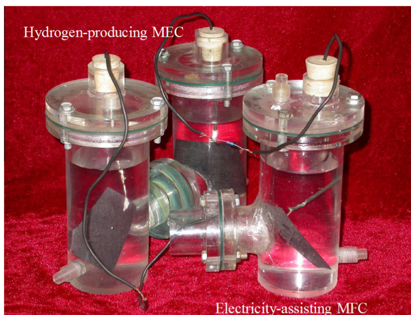
Figure 16 Laboratory-scale prototype of the MEC–MFC-coupled system.
