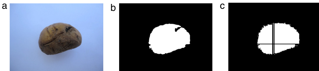
Fig. 13. Sample images for size sorting. (a) Original image, (b) binarized image, (c) size detecting.
