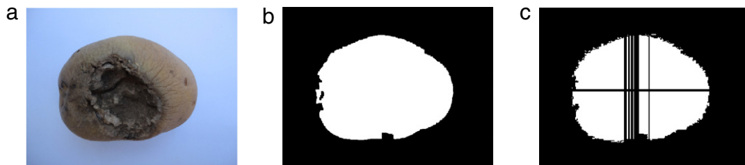
Fig. 15. Sample images for size sorting. (a) Original image, (b) binarized image, (c) size detecting.
