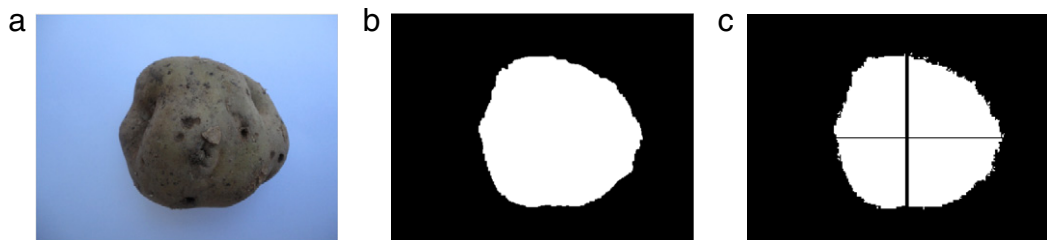
Fig. 14. Sample images for size sorting. (a) Original image, (b) binarized image, (c) size detecting.
