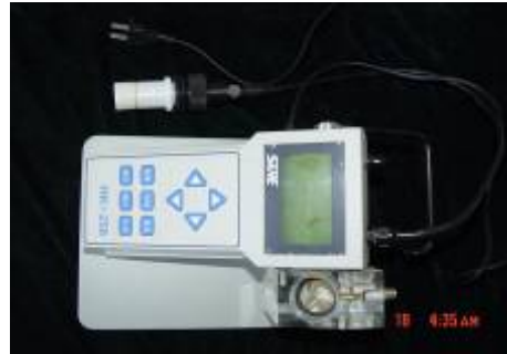
Fig.1. 1 oxygen electrode, 2 electrode cap, 3 electrode signal line, 4 entrance of circulation detection pool, 5 exit of circulation detection pool, 6 circulation detection pool, 7 catheter, 8 catheter platform, 9 host
