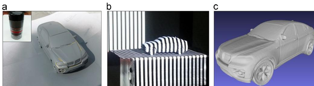
Fig. 11. A process of making a mock-up of car: (a) painting with a diffuse spray, (b) acquiring a 3D model using a structured-light 3D scanner, and (c) 3D mesh model of a car  $|V| = 100k$ .
