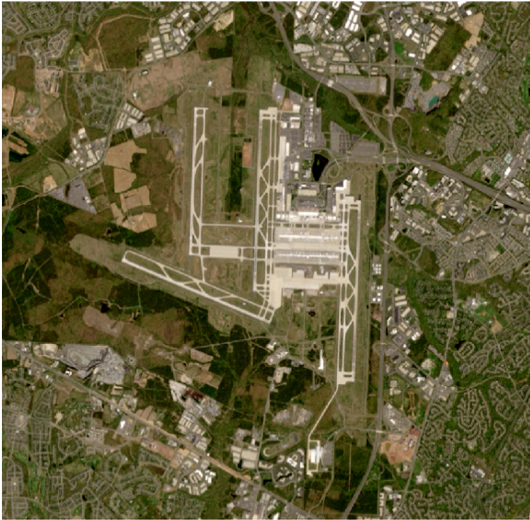
Fig. 2. Full resolution depiction of Dulles Airport, in Virginia just west of Washington, DC, extracted from the OLI surface reflectance image (Fig. 1a). The OLI panchromatic band (0.500–0.680 \mu\text{m} ) has been used to sharpen the resolution of the red, green and blue bands. A region of 9 km \times 9 km is shown.
