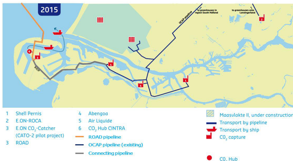
Fig. 3. Overview of CO 2 network in Rotterdam region (blue/OCAP is existing, gray is connection pipeline, and orange is new offshore pipeline to CO 2 storage site linked to ROAD project).
