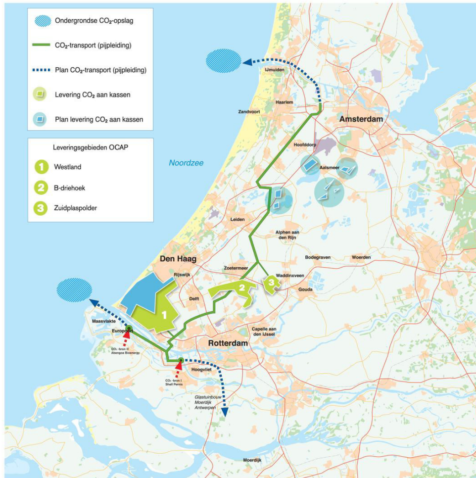
Fig. 2. OCAP pipeline (in green) with possible extensions (in blue).
