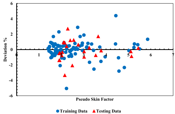
Fig. 10. Relative error distribution of the obtained outputs from LSSVM model versus corresponding pseudo skin factor data points.
