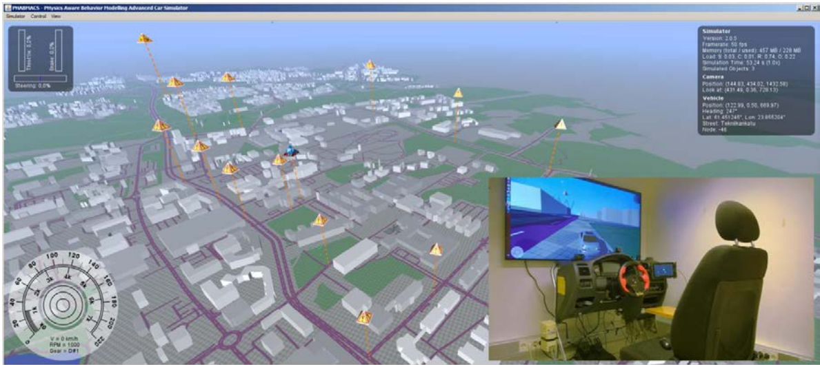
Fig. 3. City model and hardware in the loop simulator for DENM delivery.
