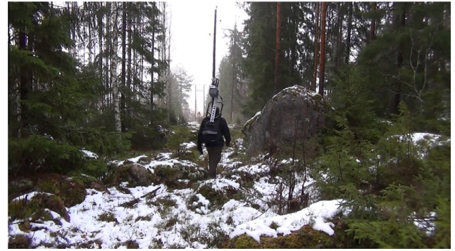
Fig. 5. Scanning of a power line corridor with a backpack PLS laser scanning system (FGI AkhkaR2).
