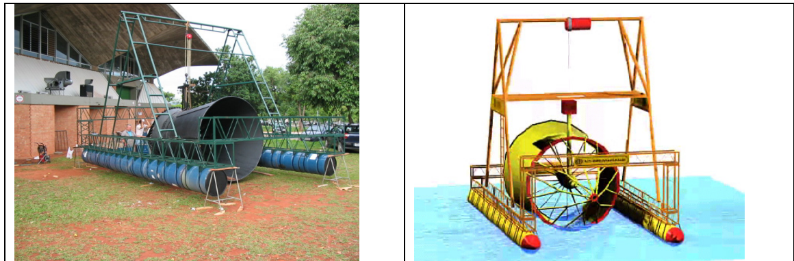
Figure 2. Anchoring and floating system for hydrokinetic turbines.
