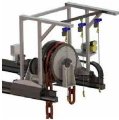
Figure 7-1 – The movable windlass is a concept designed to operate multiple mooring lines within the same area. Normally, one windlass skids along a special foundation to operate one mooring line at a time [48]
