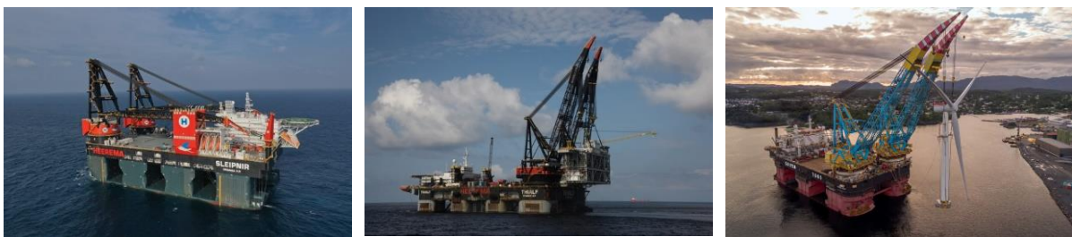
Figure 5-6: Exemplary selection of semi-submersible crane vessels; Left: Heerema Sleipnir [Source: Heerema], Middle: Heerema Thialf [Source: Heerema], Right: Saipem 7000 [Source: Saipem].
