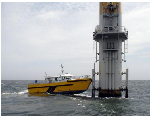
Figure 5-39. CTV in crew transfer manoeuvre [Source: [28]].
