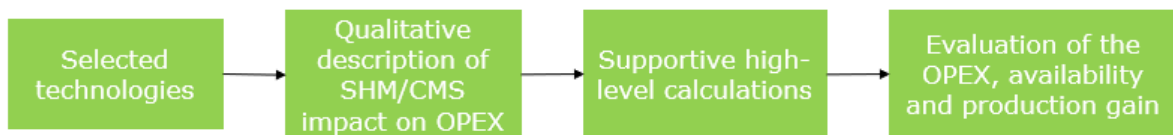
Figure 5-1: Workflow for the identification of the cost reduction potential of the monitoring systems suitable for floating offshore wind
