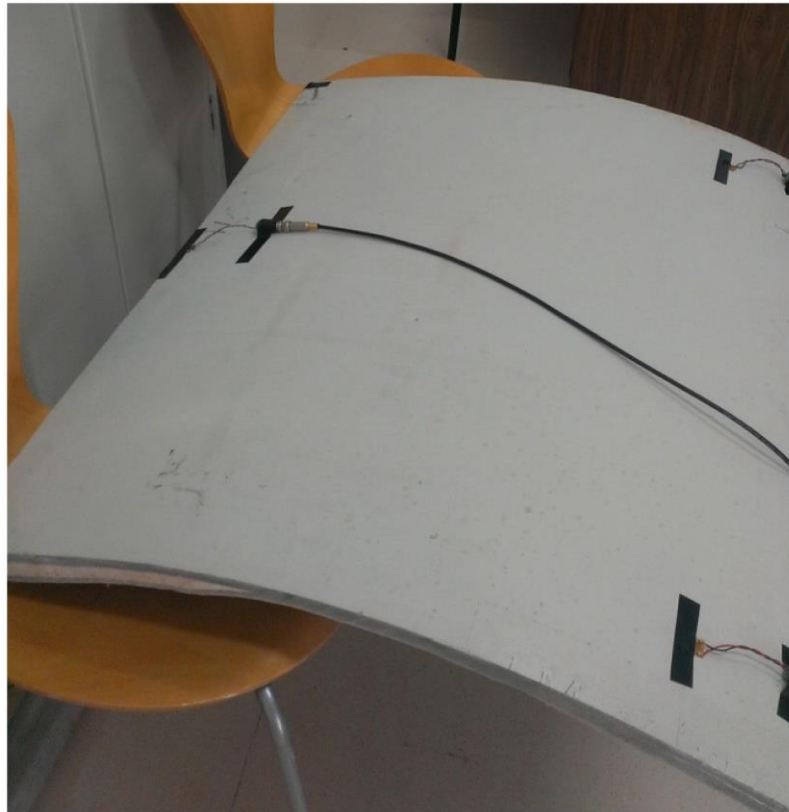
Figure 4-5. Blade section with acoustic emission sensors [17].
