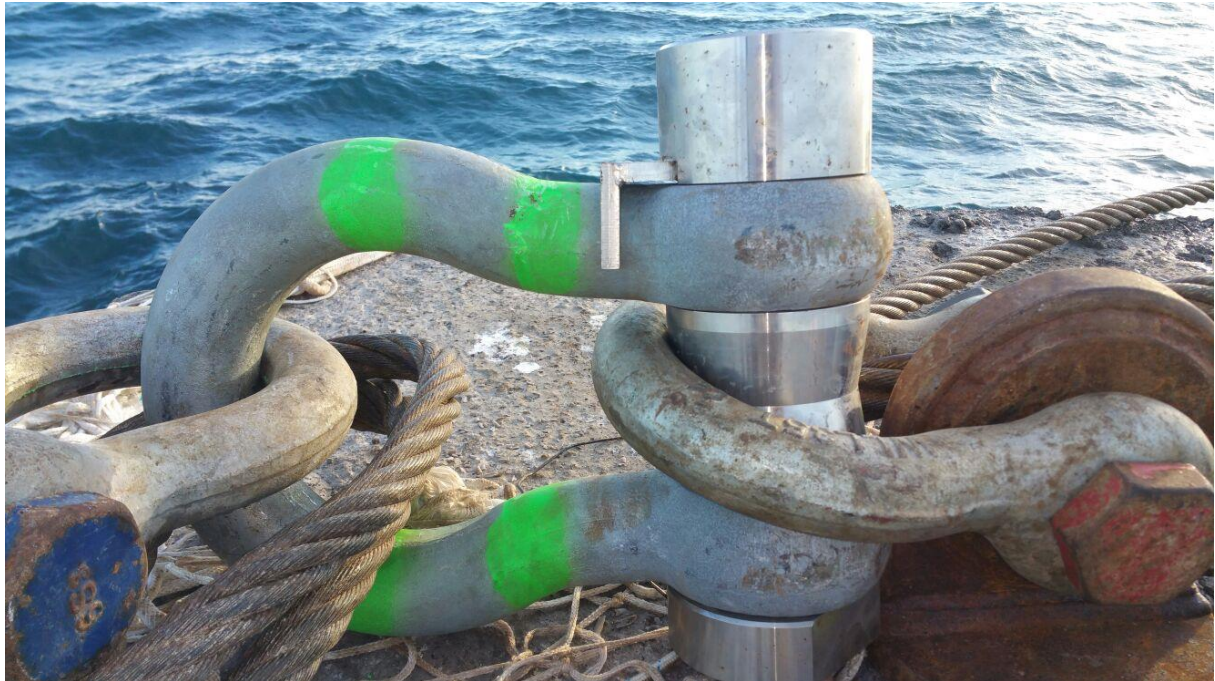
Figure 4-6. 75 ton load shackle [21].
