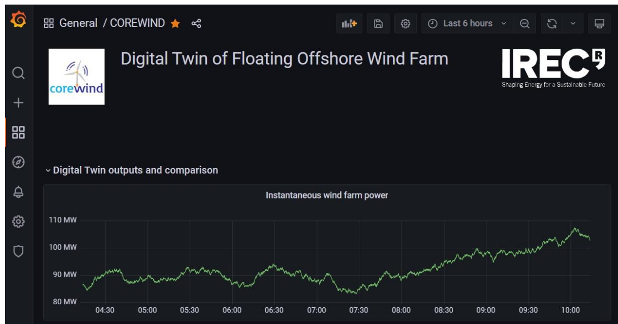
Figure 5-9. Example of the visualisation platform developed for the digital twin.
