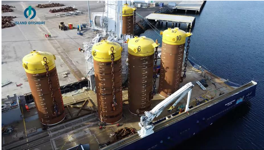
Figure 5-1: Example of Suction Anchor Piles with temporary lower chain segment positioning [Source: Island Offshore].
