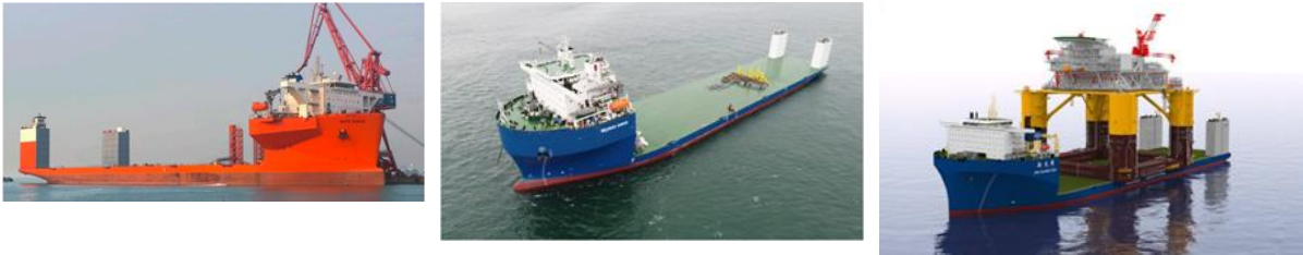
Figure 5-6: Exemplary semi-submersible heavy transport vessel White Marlin [Source: Boskalis], semi-submersible HTV Seaway Swan [Source: Seaway 7], semi-submersible HTV Xin Guang Hua [Source: Cosco Heavy Transportation].
