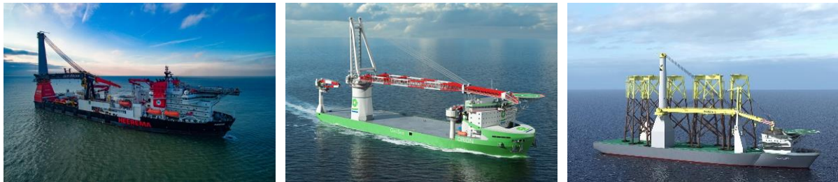
Figure 5-2: Exemplary monohull heavy lift crane vessels; Left: Heerema Aegir [Source: Heerema], Middle: Deme Orion [Source: Deme], Right: Boskalis Boka Lift 2 [Source: Boskalis].
