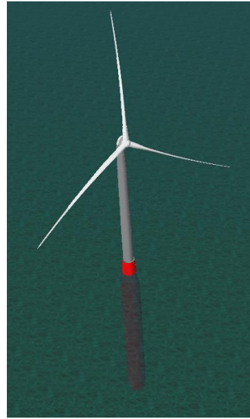
Figure 6-4: Illustration of the OrcaFlex model of the Windcrete spar equipped with the IEA 15 MW reference wind turbine [Source: Ramboll].
