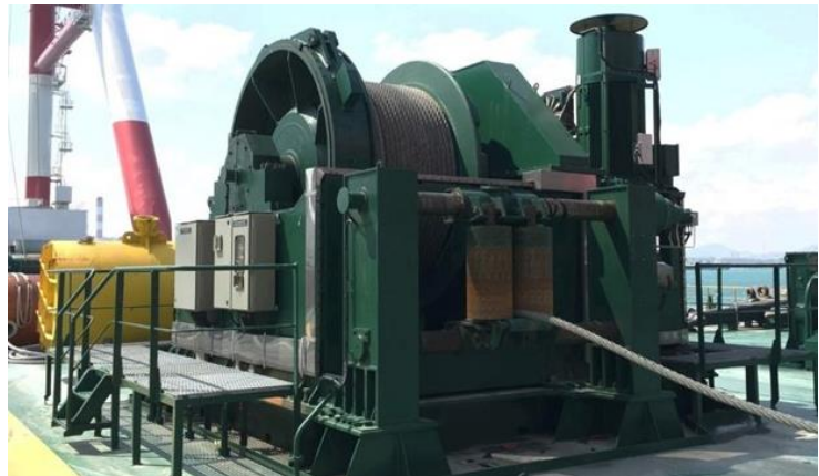
Figure 7-2 – Example of Mooring Winch [48]
