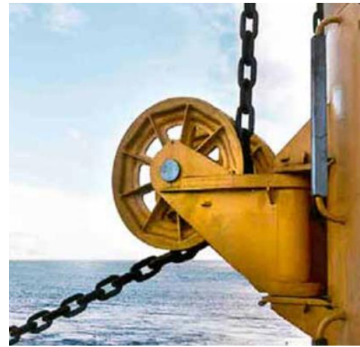
Figure 7-4 – View of Fairlead/ Examples - Pusnes eccentric chain fairlead from Mac Gregor [48]
