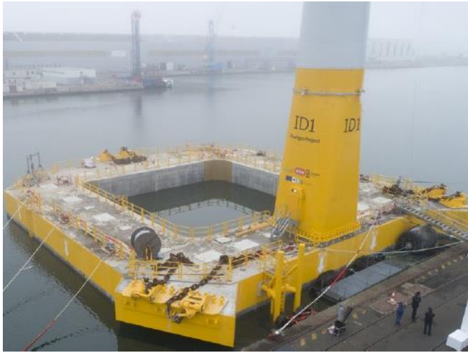
Figure 7-3 – View of floaters / Examples - Extract from reference [15] to illustrate floater / mooring interface for Floatgen
