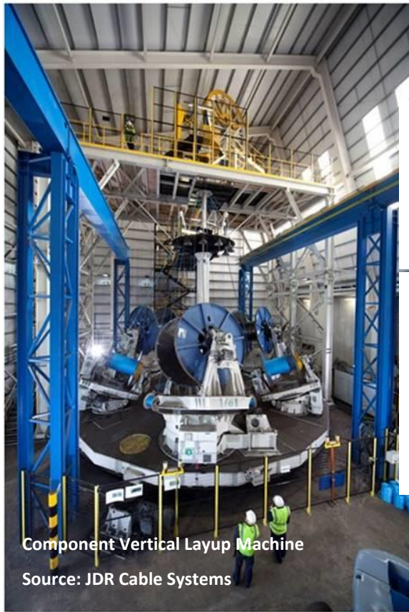
Figure 3.1-3 – Component layup operation and theory
