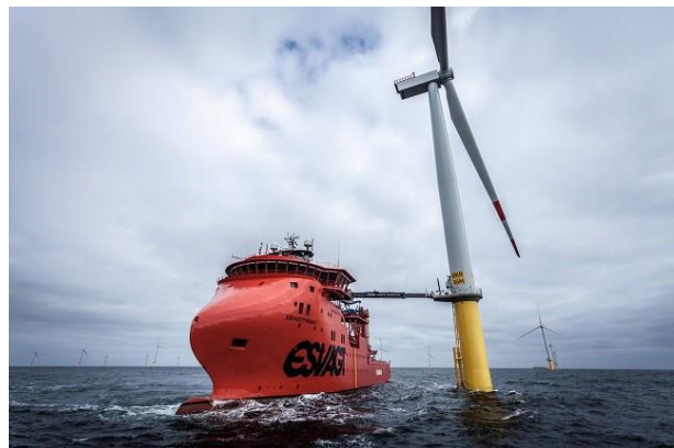
Figure 5-40. SOV in crew transfer manoeuvre [Source: Esvagt Faraday].
