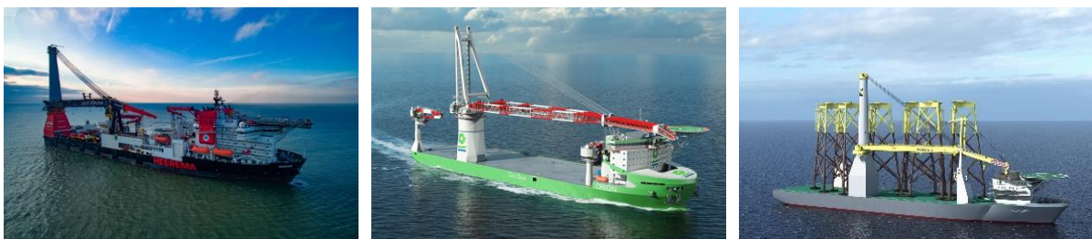
Figure 5-7: Exemplary selection of monohull heavy lift crane vessels; Left: Heerema Aegir [Source: Heerema], Middle: Deme Orion [Source: Deme], Right: Boskalis Boka Lift 2 [Source: Boskalis].
