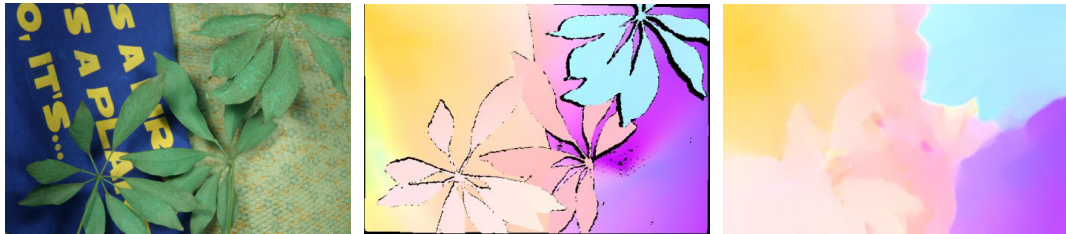
Figure 2.6. First frame of the “Schefflera” sequence from the Middlebury benchmark, the ground truth flow field (the dark regions correspond to occlusions and are excluded from evaluation), and the estimated flow field by the Combined Local and Global (CLG) method [38]. Though achieving good result on the “Yosemite” sequence (cf. Figure 2.5), The CLG method fails to recover the sharp motion boundaries and the occlusion regions.
