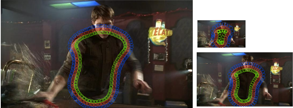
FIGURE 5. Contour-based likelihood features. HOG descriptors are computed at contour points (red), inside (green) and outside the contour (blue) in a 3-level pyramid.
