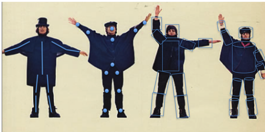
FIGURE 15. Human pose estimation. Output can be a set of sticks, body joints, or values for model variables of location and rotation of boxes or 3D shapes.
