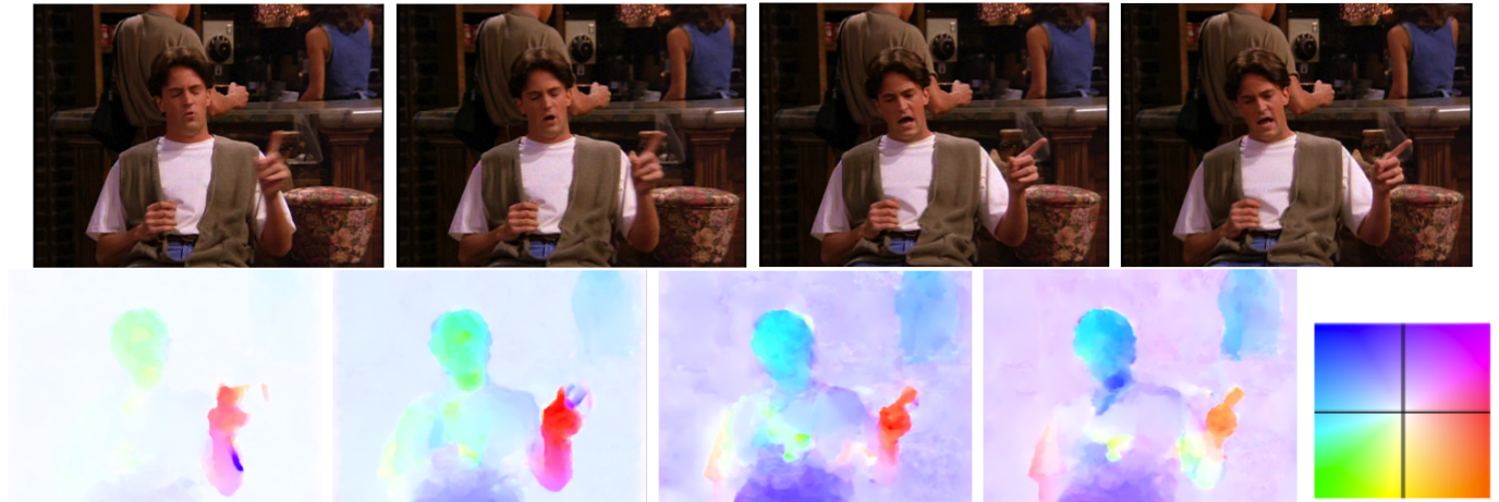
FIGURE 1. Optical Flow. The second row shows the forward optical flow of the sequence of frames in the first row. In the optical flow images the hue corresponds to the direction as indicated in the image on the right. The saturation corresponds to flow magnitude.
