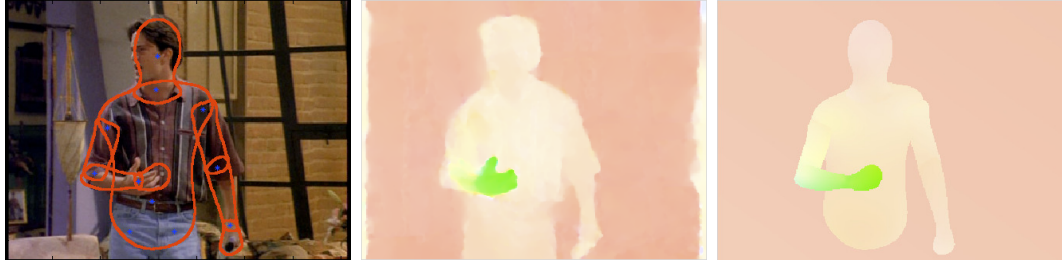
FIGURE 3. Puppet flow. (left) Frame with overlapped a DS model; (center) dense optical flow; (right) puppet flow.
