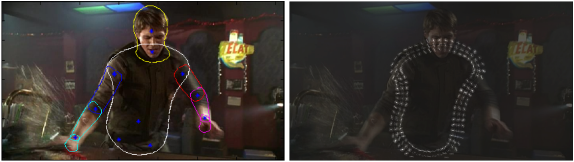
FIGURE 3. HOG descriptors are steered to the contour orientation. (a) DS annotation. (b) HOG visualization.
