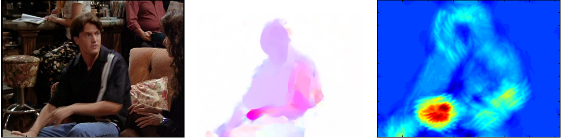
FIGURE 6. Hand detection. Example of output from the hand detector trained on optical flow. Image (left), optical flow (center), and hand probability map defined from running a flow-based hand detector on the flow (right).
