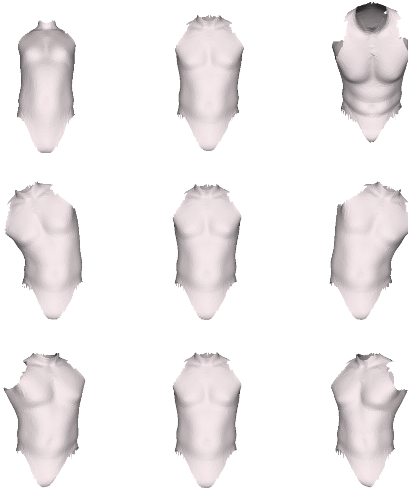
FIGURE 5. Pose-dependent part deformation. An example of the torso PCA model is shown (first three principal components from top to bottom). The center mesh in each row is the mean shape and the left and right meshes correspond to \pm 3 standard deviations from the mean.
