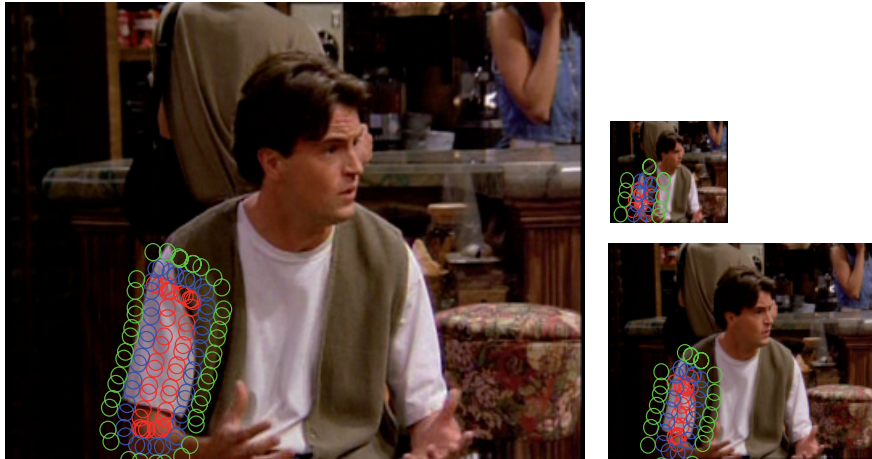
FIGURE 5. Contour-based likelihood features. HOG descriptors are steered to the contour orientation and computed at contour points (blue), inside (red) and outside the contour (green) in a 3-level pyramid.
