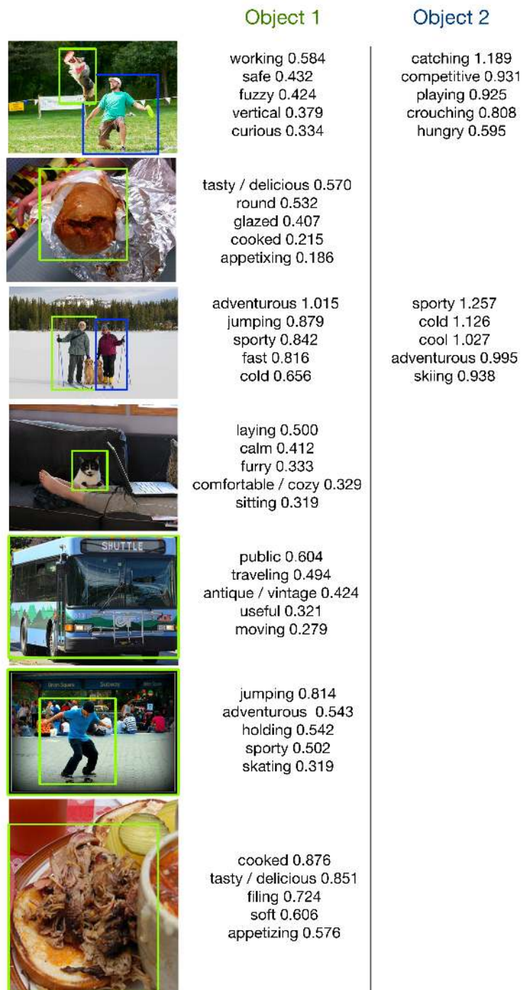
Figure 3.8: Example Attribute Classifications . In the figure above, images from the MS COCO dataset that were not part of the MS COCO Attributes set are shown. The objects are identified with either a green or blue bounding box. Beside the test images, 5 of the most confident attribute detections for that bounding box are listed along with the SVM confidence score. The attribute classifiers used for this figure correspond to the SVM classifiers in Fig. 3.7. This figure is a qualitative example of how detected MS COCO Attributes can give a deep and broad description of the context of the object instance.
