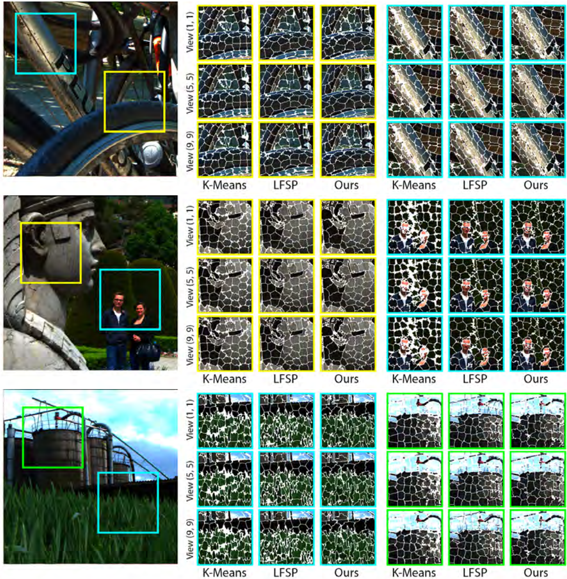
Figure 5.6: Superpixel segmentation boundaries and view consistency for the k-means baseline, LFSP [127], and our method. Disparity maps for LFSP and k -means were calculated using the algorithm of Wang et al. [107, 108]. We include six light fields from the EPFL Lytro light field dataset [80], with three more in Figure 5.7. Our superpixels tend to remain more consistent over view space, which can be easily seen as reduced flickering in our supplementary video. Note: Small solid white regions appear when superpixels are enveloped by the boundary rendering width. k -means tends to have more of these regions which helps it increase boundary recall, but this behavior is not useful for a superpixel segmentation method.
