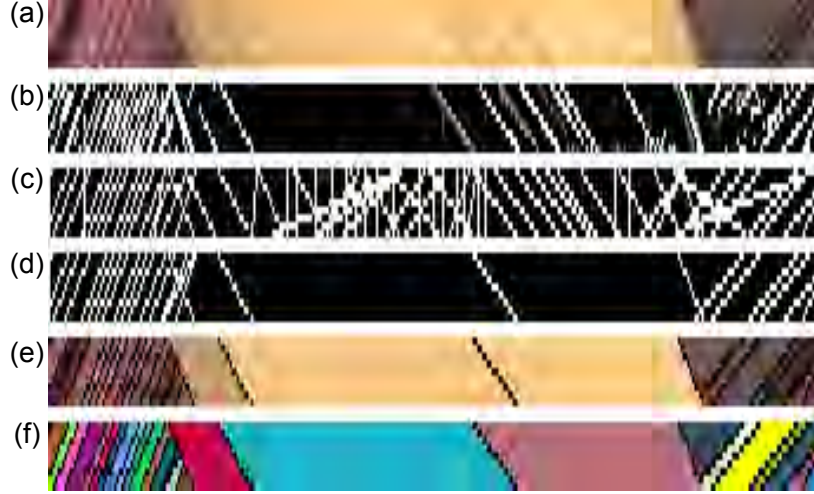
Figure 4.5: From top to bottom: (a) Input EPI. (b) Edge confidence map C from Sec. 4.1 (c) Parametric lines \mathcal{L} fit to C . As we do not threshold, faint edge lines are visible along with some outliers. (d) Outliers are robustly removed via spatial neighbor statistics, depth, and edge confidence weights. Note: remaining overlapping lines represent occlusions. (e) & (f) Line pairs are matched in an occlusion-aware manner to form angular segments. Note: The EPIs have been stretched vertically for viewing; input is 9 views.
