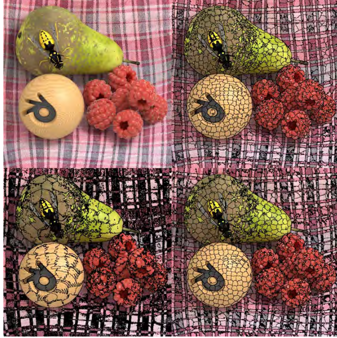
Figure 5.1: Light field superpixel comparison for the central view. Top left : Input scene. Top right : Our method. Bottom left : k -means on (x, y, d, L^*, a^*, b^*) with disparity maps computed by Wang et al. [107, 108]. Bottom right : LFSP [127] computed with Wang et al. disparity map.
