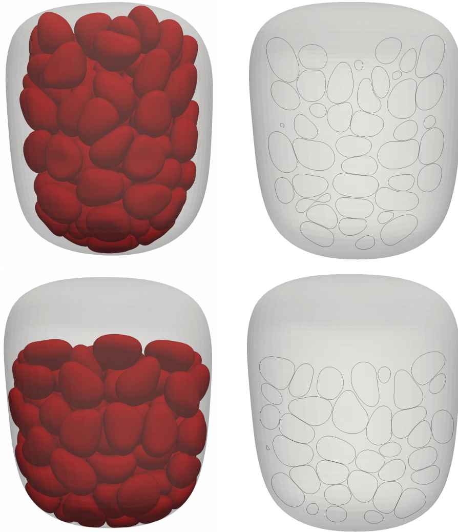
Figure 3.5: HIGH-VOLUME FRACTION SEDIMENTATION DUE TO GRAVITATIONAL FORCE.. The initial configuration (top figures) has a volume fraction of 47%. As the cells sediment to the lower part of the domain (bottom figures), the local volume fraction of the final state in this lower part of the domain is around 55%. Shown on the right side are slices through the center of the domain together with the RBC boundaries in the initial and final configuration. The full simulation video is available at https://vimeo.com/329509435 .
