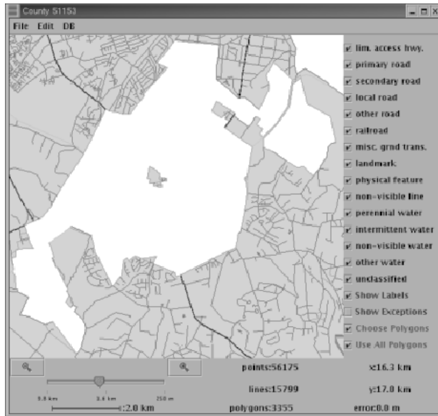
Figure 3.3: Prince William County, Virginia. Contains a hole, islands inside the hole, and a strip dividing the hole.
