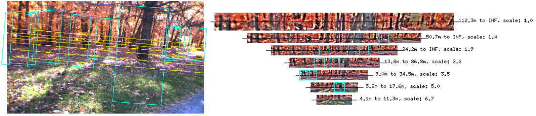
Figure 4.5: The input image at left has been systematically cropped, leveled and subsampled to yield each pyramid row seen to the right. The bounding boxes demonstrate the effectiveness of the normalization: trees that are different scales in the input image are similarly scaled in the pyramid.
