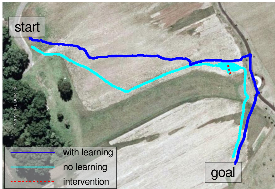
Figure 6.14: This experiment compared the long-range system with the CMU baseline software. The fourth course was much longer, and had a large tall-grass obstacle (the green terrain in the satellite picture was impassable tall grass when the test occurred). The short-range baseline system drove straight to the obstacle before turning and navigating around it, whereas the long-range system detected the barrier and planned around it, jumping onto a paved path for a short distance.
