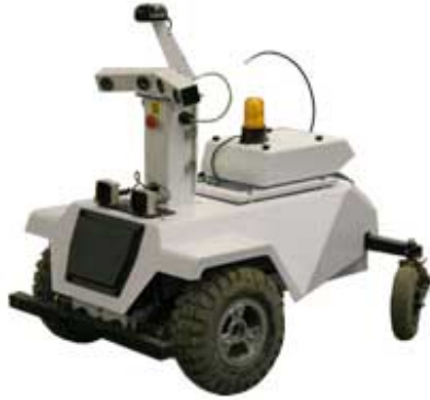
Figure 4.3: The LAGR mobile robotic vehicle, developed by Carnegie Mellon University’s National Robotics Engineering Center. Its sensors consist of 2 stereo camera pairs, a GPS receiver, and a front bumper.
