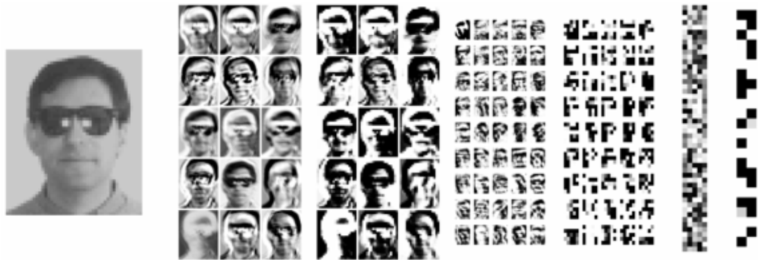
Figure 3.4: Internal state of the convolutional network for a particular example.
