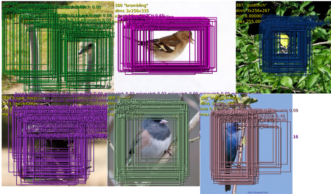
Figure 4.11: Examples of bounding boxes produced by the regression network , before being combined into final predictions. The examples shown here are at a single scale. Predictions may be more optimal at other scales depending on the objects. Here, most of the bounding boxes which are initially organized as a grid, converge to a single location and scale. This indicates that the network is very confident in the location of the object, as opposed to being spread out randomly. The top left image shows that it can also correctly identify multiple location if several objects are present. The various aspect ratios of the predicted bounding boxes shows that the network is able to cope with various object poses.
