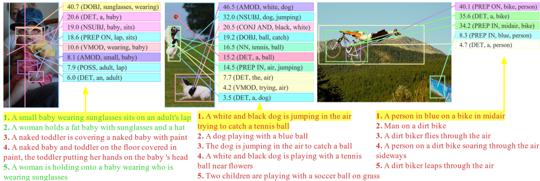
Figure 4: Qualitative Image Annotation results. Below each image we show the top 5 sentences (among a set of 5,000 test sentences) in descending confidence. We also show the triplets for the top sentence and connect each to the detections with the highest compatibility score (indicated by lines). The numbers next to each triplet indicate the matching fragment score. We color a sentence green if it correct and red otherwise.
