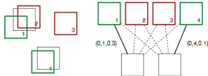
Figure 5. Illustration of the matching of ground-truth instances (black) to accepted (green) and rejected (red) candidates. Matching should respect both precedence (1 vs 2) and localization (4 vs 3).
