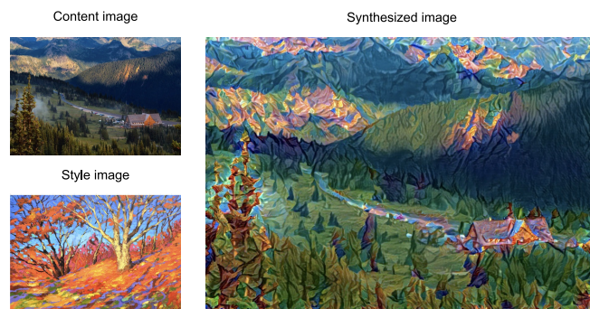
Fig. 14.12.1 Given content and style images, style transfer outputs a synthesized image.
