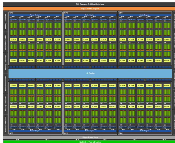
Fig. 13.4.8 NVIDIA Turing architecture (image courtesy of NVIDIA)
