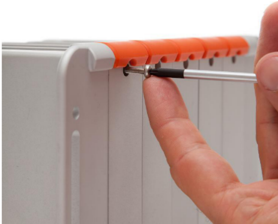
Illustration 301: Module-Backplane screw connection
