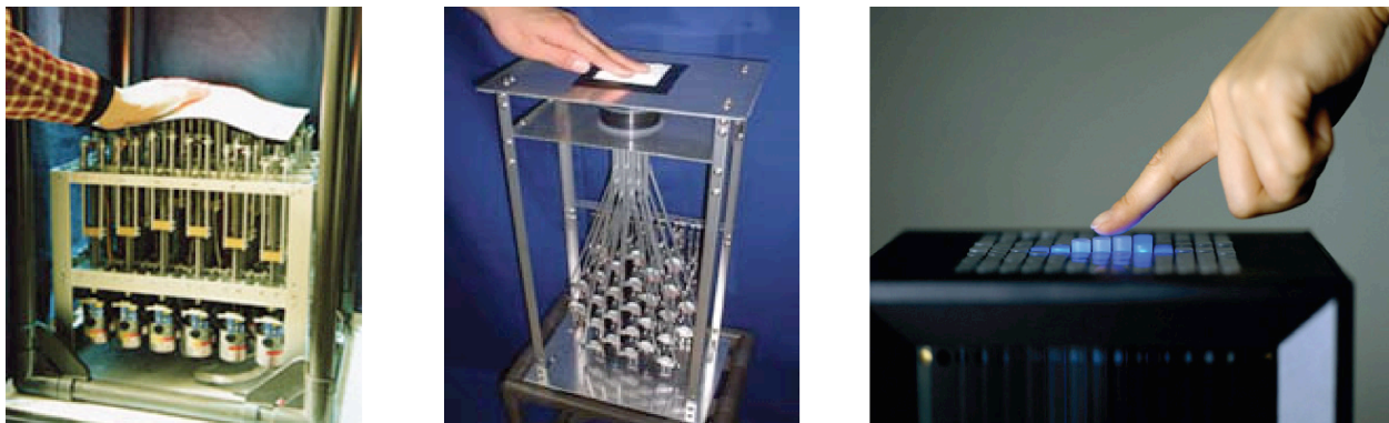
Fig. 10 - 2.5D Shape Displays: FEELEX 1 & 2 and Lumen
