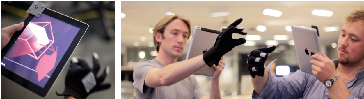
Fig. 14 - T(ether), a collaborative system to interact with volumetric data using gestures
