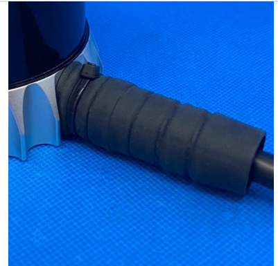
Fig. 1.11: Final Connector Sealing Step 3
