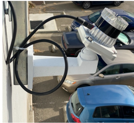
Figure 1.17: Typical Drip Loop
