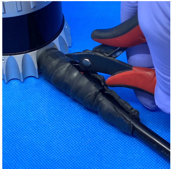
Fig. 1.16: Removal of self-vulcanizing tape (Finish)
